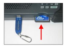
The USB thumb drives may be installed or removed at any time while the product is in use. However, the Compact Flash memory must be installed in the TALAN on startup to be properly recognized and accessed.
