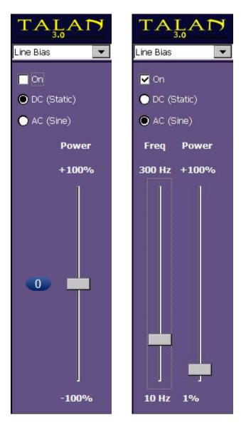
It is highly recommended that the rotary dial be used to adjust the power level of the Line bias function. The rotary dial provides a much finer control, while the stylus may provide quick, large, jumps in voltage. You should be careful not to put too much voltage on a line.
