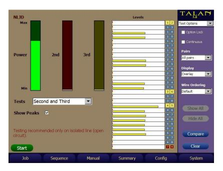
To determine the proper pair with the tap, the transmit power is manually decreased until only the true pair shows an NLJD response.
