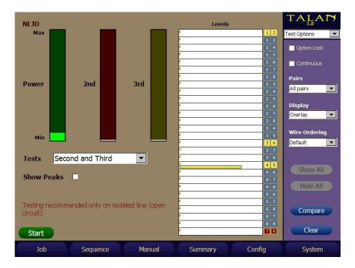
In the next example, there is a serial tap only on conductor number 8. Therefore, only combinations that contain conductor 8 will get a response.
