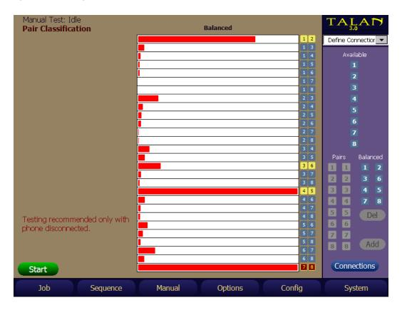
After reviewing the balanced line data, you should manually define the combinations of balanced pairs by selecting them in the Define Connections dashboard. Tap the connector numbers that make up the pair and select Add to define the pair as a balanced pair. Once the balanced pairs have been defined, all other test screens will display the balanced pairs with a yellow background.
