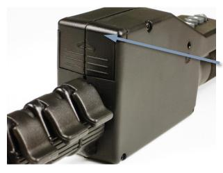
The power source is a 9 V alkaline battery. There is a sliding door that is used to retain the battery. Insert the battery in the correct orientation as indicated by the label inside the compartment.
