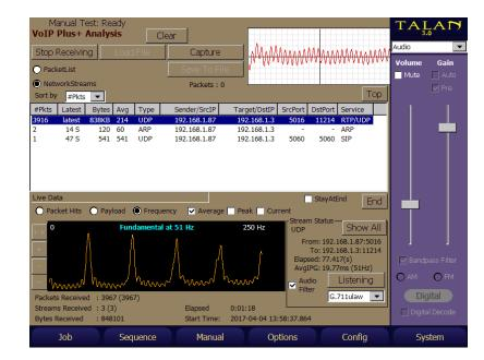
An Audio Filter can be enabled to improve the sound of the audio, if it is indeed audio.
