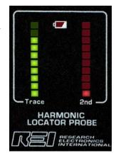
Figure 5 Combination Mode with no device detected
