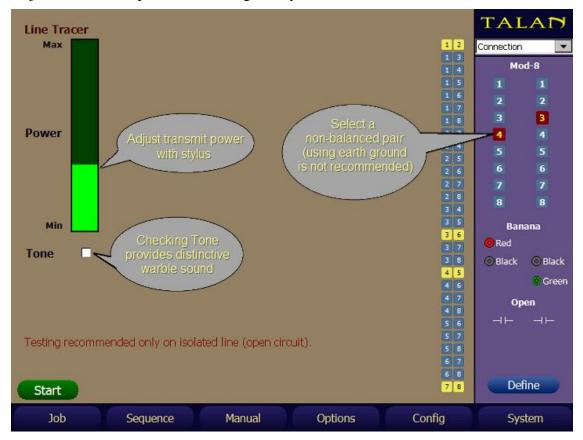
5. Adjust the transmit power level using the stylus.
