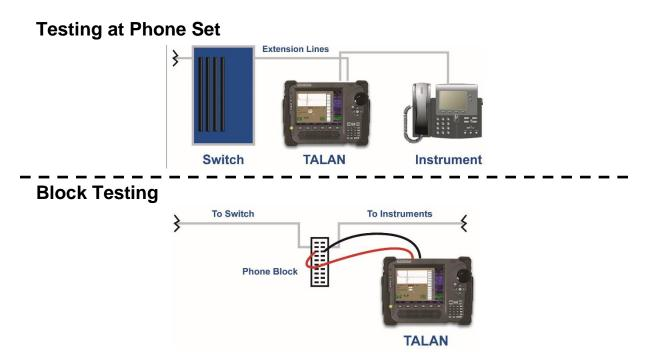
It is important to understand that prior to interrupting the phone line you should first verify that there is no audio passing down the line. Therefore, regardless of where you test the line, you should first use the banana plugs, connect to the main audio pair and test for audio. This is often easier at an intermediate block. Then, it is recommended that the user start testing at the phone set. For the remainder of this document, it is assumed that the testing is performed at the phone set.
