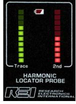
Figure 4 Combination Mode with device detected
