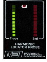
The Tracing Mode utilizes a 225 kHz signal that is generated by the TALAN and is injected into the wire to be traced. Enabling Tone on the TALAN adds a tone modulation to the signal which may be discernable before seeing a change in the bargraph.
