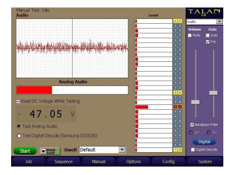
It is also interesting to note that the audio levels are basically the same for the combinations that contain audio. This is because the strength of the digital system is not indicated through the digital demodulation process. In other words, a weak digital signal and strong digital signal will basically result in the same analog audio level after the demodulation.
