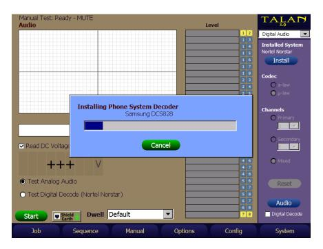
In the Digital Audio dashboard, Channels indicates which side of conversation is being demodulated. Select Mixed in order to hear both sides of the phone conversation, Primary to hear only the handset, or Secondary to select the audio coming from the switch. To listen to normal analog audio, Digital Decode should be unselected.
