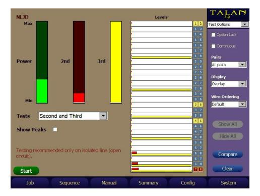
In the next example below, there is an electret microphone that is placed on an unbalanced pair combination of 1:3. You can see a strong 2<sup>nd</sup> harmonic response on many pair combinations that contain 1 or 3, and also some response on the unbalanced 2:6 pair whose conductors are balanced with 1 and 3. This is an excellent example of inductive coupling that can occur in a telephone line.
