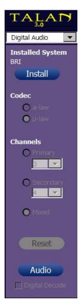
The Codec indicates the type of modulation that is used.  $\mu$ -law is used primarily in North America and Japan while a-law is prominent in the rest of the world.
