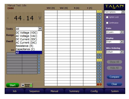
Then, select which tests to measure as shown above. It should be noted that to prevent a nonpractical test there are automatic conditions for performing some of the tests (for example, you cannot measure capacitance on a line that is terminated or powered).
