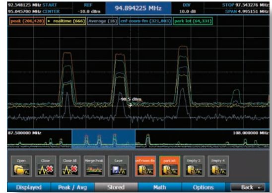
Zoom to a frequency range while continuing full peak capture
