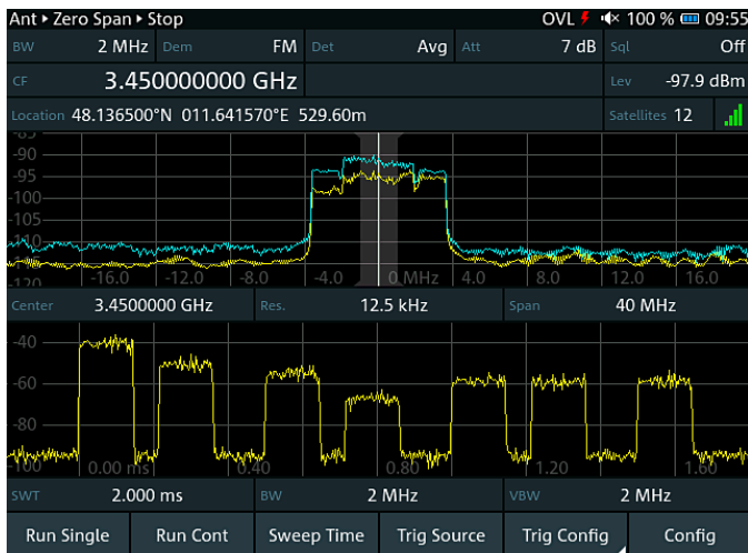
Simultaneous display of the frequency domain (top) and the time domain (bottom)
