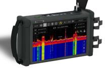
**Cached Peak** *Patent Pending* - The MESA<sup>™</sup> dynamically adjusts resolution bandwidth depending on viewed frequency span. The Cached Peak maintains multiple peak traces to reflect the appropriate frequency span and associated resolution bandwidth.
